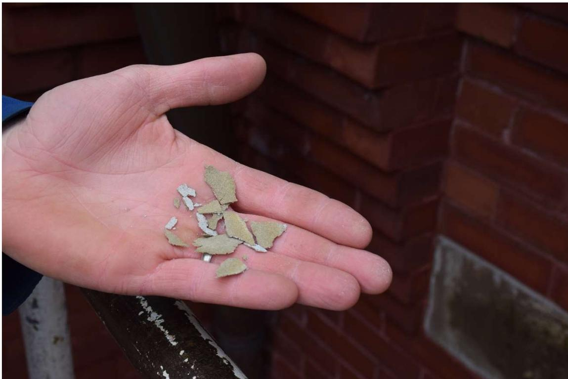
Delamination of Stone Behind Coating
